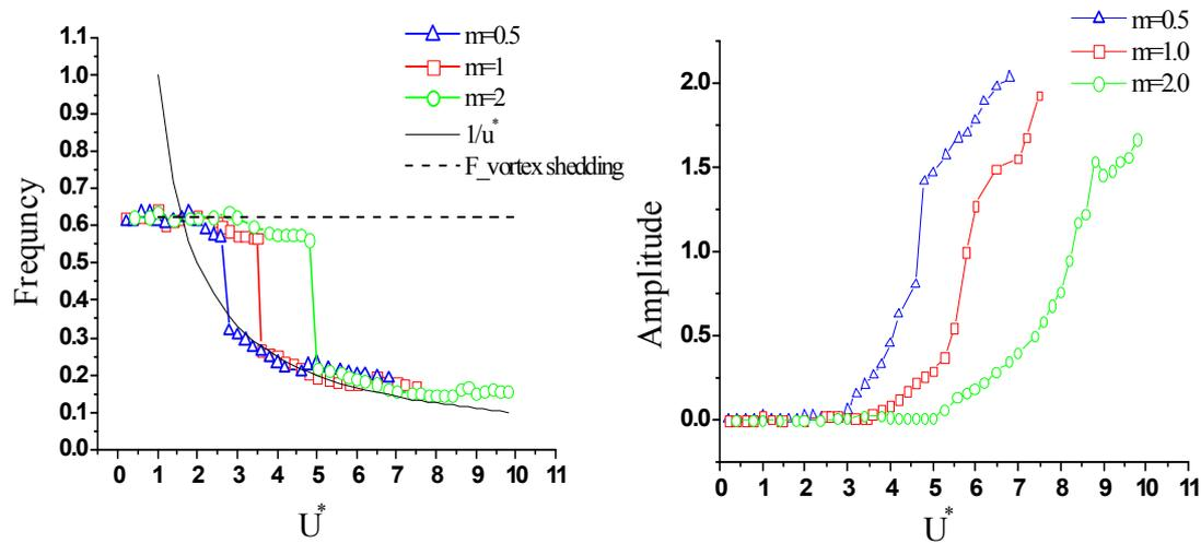
Fig. 3 Variation of the frequency and the amplitude of transverse oscillation with  $U^*$  at different mass ratio
